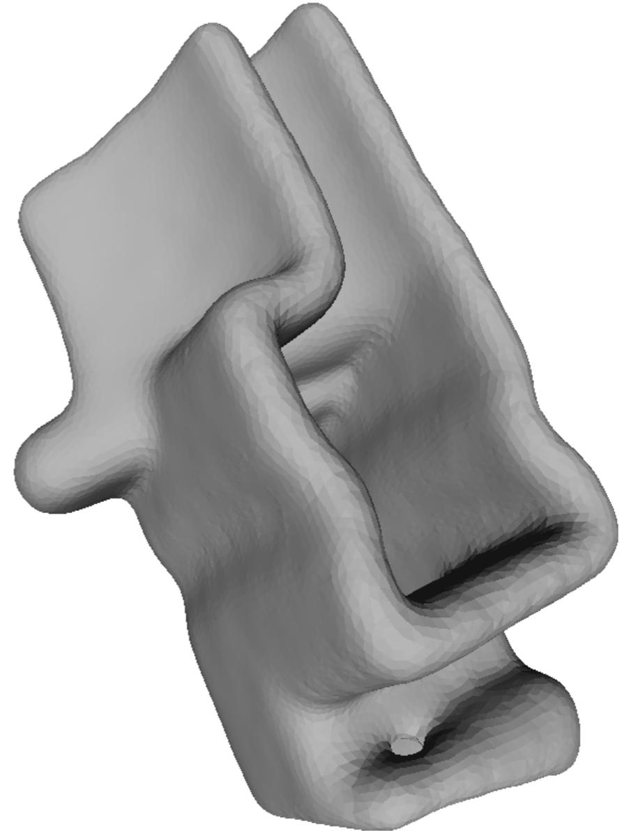
Reconstruction of an offset of a mechanical part from a noisy approximation with 10% outliers
